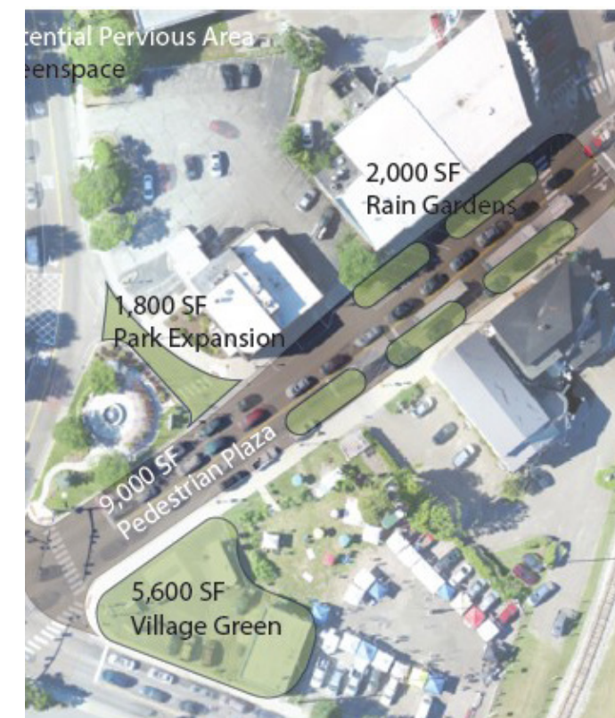
The implementation plan shows a pedestrianized Main Street with gardens designed to absorb runoff from surrounding buildings.
